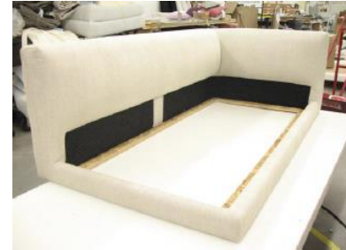
BACK BODY Ball Fibre Fill along the body.
